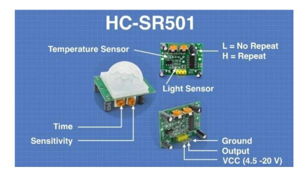
There are also two potentiometers on the board to adjust a couple of parameters:
